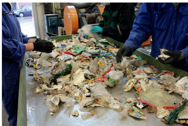
A polystyrene fraction from the German dual system of waste collection is sorted manually.
