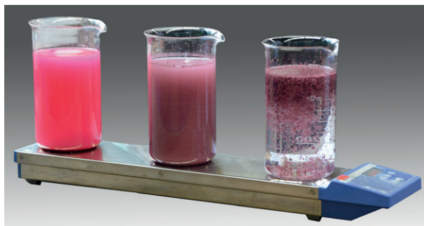
Flocculation of microplastics (left: suspended microplastics; middle: the flocculation process; right: microplastic flakes rising to the surface).
