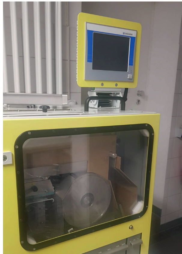
A modified electrostatic plastic separator separates microplastics from sediments and arable soils.
