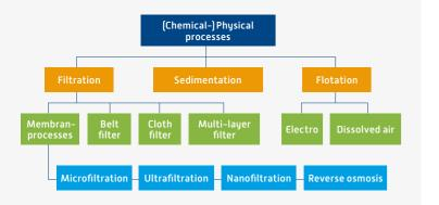
Identification of input pathways has shown that microplastics can enter wastewater along the complete value chain (production - processing - shipping). Filtration, flotation and sedimentation processes are best suited to removing them from wastewater. The efficiency of these processes could be significantly improved by specially developed flocculants.
