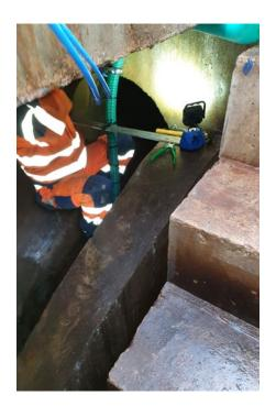
Suitable sampling sites, such as this inlet of an underground storm water basin, are not always easily accessible.
