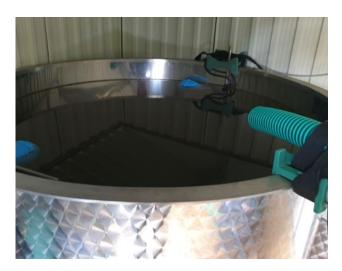
Stainless steel collection container (1,000 L) for large sample volumes during rainy weather used to obtain a sufficient volume of microplastics.
