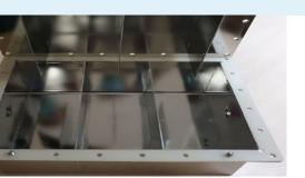
With the aid of a sedimentation box it is possible to sample over long periods of time and thus to separate larger quantities of solids (suspended matter) from the water phase. Its design leads to an abrupt enlargement of the cross-sectional area through which the water flow passes, which leads to a reduction of the flow velocity and thus to the sedimentation of (microplastic) particles.
