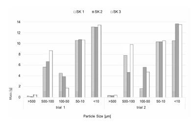
After fractionating, it is possible to depict the measures of particles deposited in sedimentation boxes according to their size distribution. Fig.: © UBA
