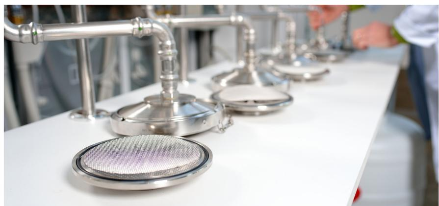
The wash water is filtered using a filter cascade (1.5 mm - 5µm pore size) and fibers are collected and analyzed by size.
